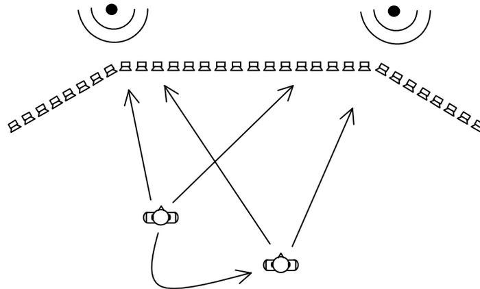
**Fig. 7 - Realization of a virtual scene presenting a compatibility with stereophony 2-0.0 by means of spherical waves. The “sweet spot” arise: according to the position of the listener, the perceived effect varies.**
