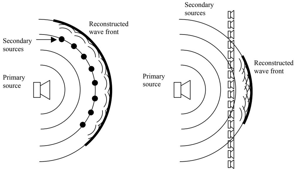
**Fig. 3 – On left, the Huygens's principle of construction. On right, the principle of construction applied to sound fields reproduction by means of practical and real sources.**
